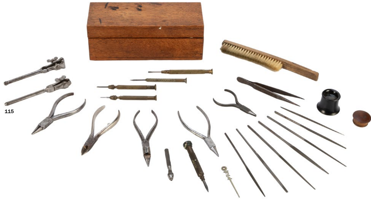
115. MASKELYNE, John Nevil (1839 – 1917). J.N. Maskelyne's Toolbox and Tools. A small oak case with hinged lid containing twenty-three tools as commonly used by a watch or clockmaker or repairman, among them two small clamps (one stamped "France"), a quantity of rasps/files, round and flat pliers, small cutters, a rough brush, a heavy set of metal tweezers, and a loupe, together with a small turned wooden box containing parts for watches, and a fancy minute hand from a vintage clock. The largest item approximately 7 ¼" in length. Most tools in good working condition, though showing considerable wear, with the toolbox itself (8 x 3 x 3") cracked and worn but solid and intact. A framed letter of provenance accompanies the toolbox. Dated October 1985, addressed to John Salisse, and signed by four members of the Maskelyne family, it states, "This small tool-box was once owned & used by John Nevil Maskelyne. The members of the Maskelyne family currently resident in this country would like you to accept with affection this as a gift in gratitude for all you do to keep the family name alive." A small number of related letters and correspondence from Joan Maskelyne are also included.
